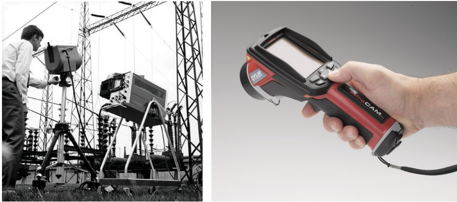
Figure 14.1 LEFT: ThermoVision® Model 661 from 1969. The camera weighed approximately 25 kg (55 lb.), the oscilloscope 20 kg (44 lb.), the tripod 15 kg (33 lb.). The operator also needed a 220 VAC generator set, and a 10 L (2.6 US gallon) jar with liquid nitrogen. To the left of the oscilloscope the Polaroid attachment (6 kg/13 lb.) can be seen. RIGHT: InfraCAM from 2006. Weight: 0.55 kg (1.21 lb.), including battery.
