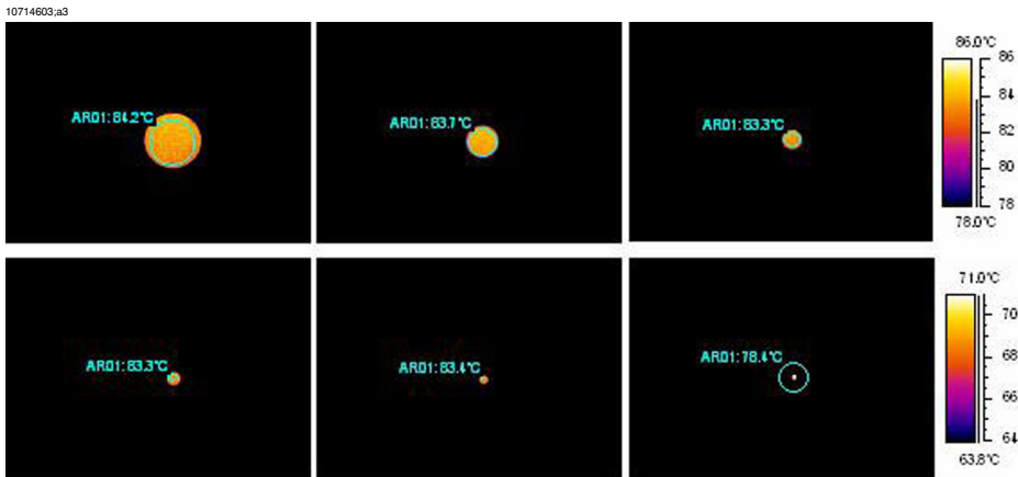
Figure 13.20 Temperature readings from a blackbody at +85°C (+185°F) at increasing distances (24° lens)
